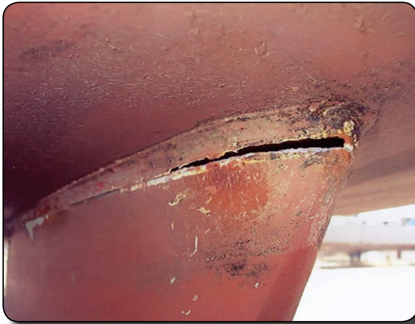
It's important to keep any chart, including a chartplotter, up to date. The damage above occurred when a sailboat struck a small concrete breakwater. The owner's GPS showed that he was right where he thought he was, but the breakwater had just been constructed (Claim #0609871).
